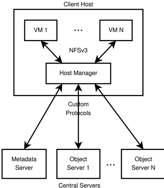
**FIGURE 3: Structure of Ventana. Each machine whose VMs use Ventana runs a host manager. The host manager talks to the VMs over NFSv3 and to Ventana’s centralized metadata and object servers over a custom protocol.**
