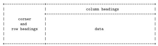
min-col-heading-width and max-col-heading-width apply to the columns in the column headings region. min-col-heading-width is the minimum width that any of these columns will be given automatically. In addition, max-col-heading-width is the maximum width that a column will be assigned to accommodate a long label in the column headings
